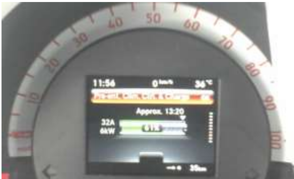
Figure 9: 15118 AC Charging With Full Power (32 Amps)
