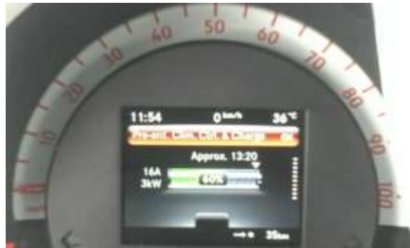
Figure 10: 15118 AC Charging With Half Power (16 Amps)
