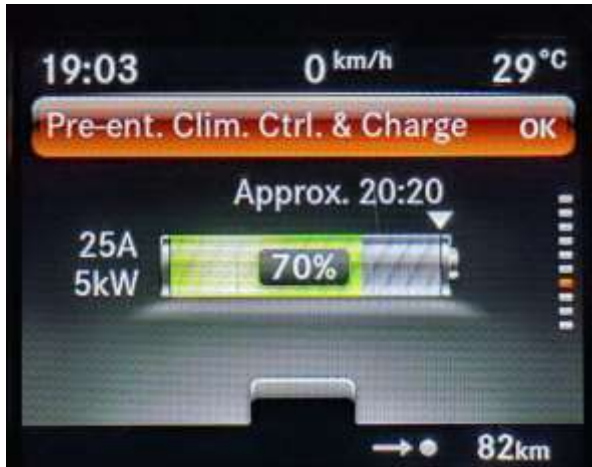
Figure 4: Close-Up of the Smart Ed Charging With 15118
