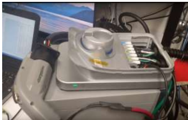
SAE J1772 charging station connector coupled to an inlet, connected to the Vector test system
