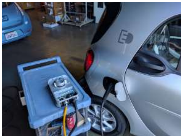
Figure 6: Prototype Home Station and Smart ED Ready for Testing in ChargePoint's Lab
