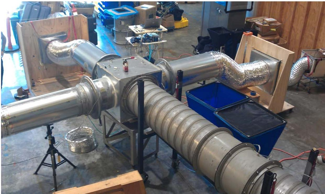
Main trunk on bottom right connecting to central plenum (center), which radiates to the three branches.
