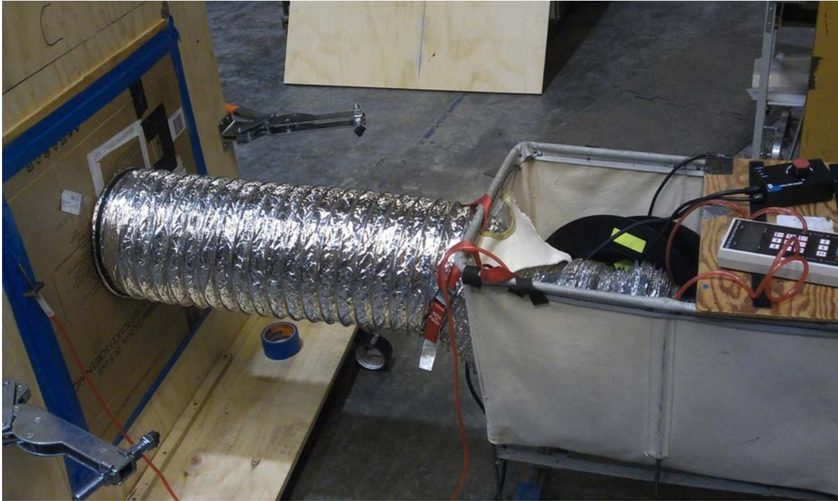
Cardboard was used to ensure that the airflow entering the grille was captured by the fan/flowmeter in card on the right. Notice that the grille is completely covered and the zero pressure tap is inserted on the left side of the cardboard.
