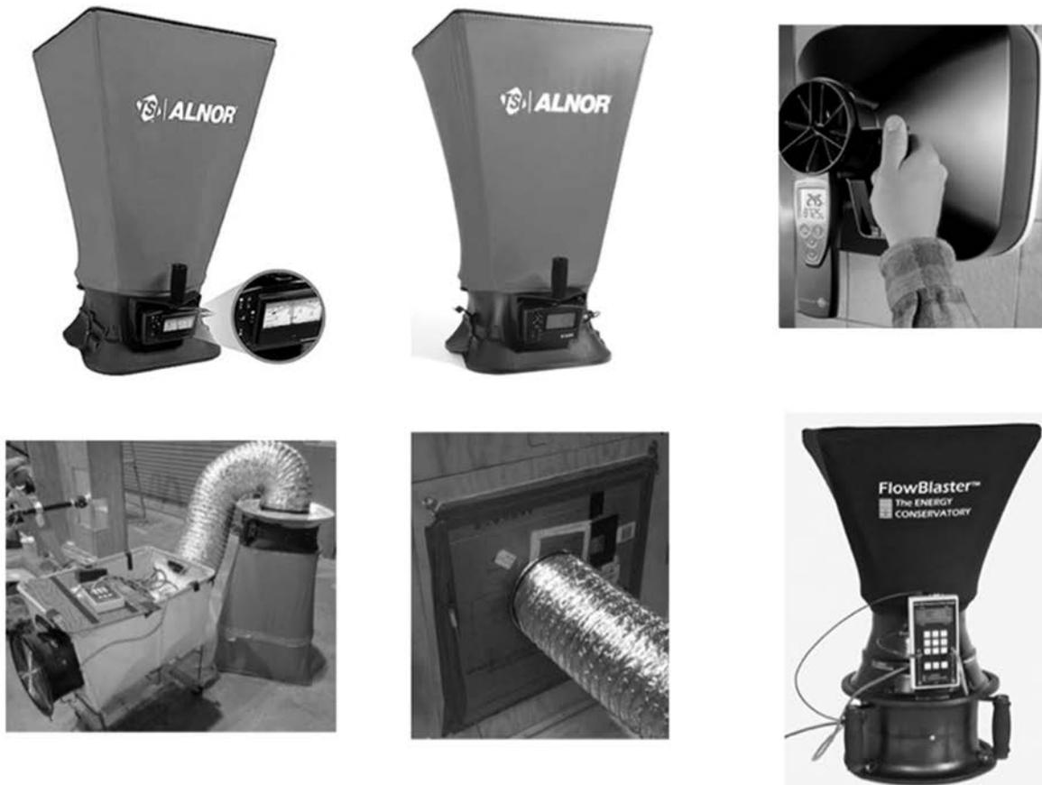
Clockwise from top left they are: TSI/Alnor ABT701, TSI/Alnor EBT721, Testo417 (shown with optional capture funnel – not used in our testing), TEC FlowBlaster, Cardboard + Fan/flowmeter, and LBNL Hybrid (uses the capture element from a traditional hood and a fan/flowmeter).
