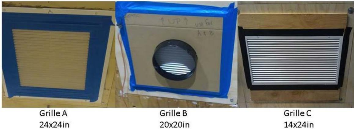
Grille A is taped off to be measured by TECFB. Grille B configured to be measured by CFF. The taping around grille C is for air sealing between the grill perimeter and the mounting plane.
